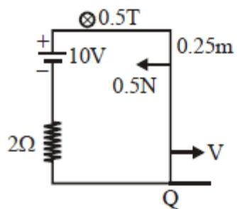
$$\text{Force } BI\ell = 0.5 \left( \frac{10 - 0.125 \text{ V}}{2} \right) 0.25 = 0.5 \text{ N} \text{ (given)}$$
