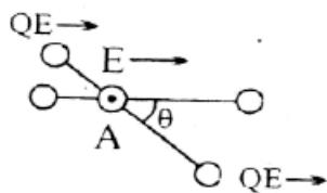
For small angular displacement  $\theta$  from equilibrium restoring torque
