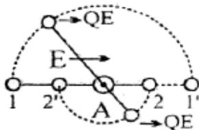
Position of maximum velocity is 1' and 2' for the balls as it is minimum potential energy position
