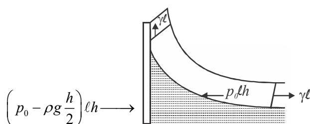
Balancing forces in horizontal direction
