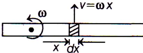
$$\Rightarrow \text{Motion emf in element} = B\omega x \cdot dx$$
