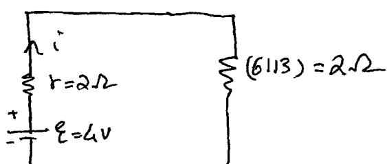
$$\text{Therefore } i = \frac{E}{R_{eq}} = \frac{4V}{2\Omega} = 1 \text{ Amp.}$$
