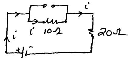
At steady state,  $t \rightarrow \infty$ , "L" acts as a short-det. Therefore from Equivalent ckt diagram  $i = \frac{2V}{20\Omega} = 0.1 \text{ Amp.}$  ✓
