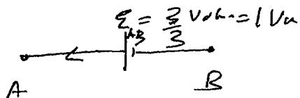
$$i = \frac{\Sigma}{R_{\text{Total}}} = \left( \frac{3}{1+2+2} \right) = 0.6 \text{ Amp}$$
