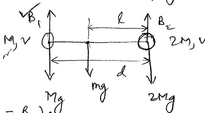
$$(Mg - B_1)(d-l) = (2Mg - B_2)l$$
