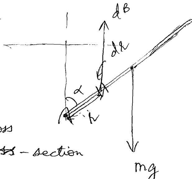
$$\begin{aligned} \therefore \text{Torque due to weight} &= mg \frac{l}{2} \cos \alpha \\ &= (\sigma A g l^2 / 2) \cos \alpha. \end{aligned}$$
