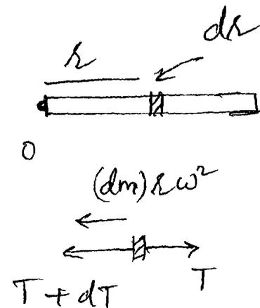
$$\text{stress} = \frac{dT}{A} = \frac{dT}{YA} = \text{strain} = \frac{dl}{l}$$
