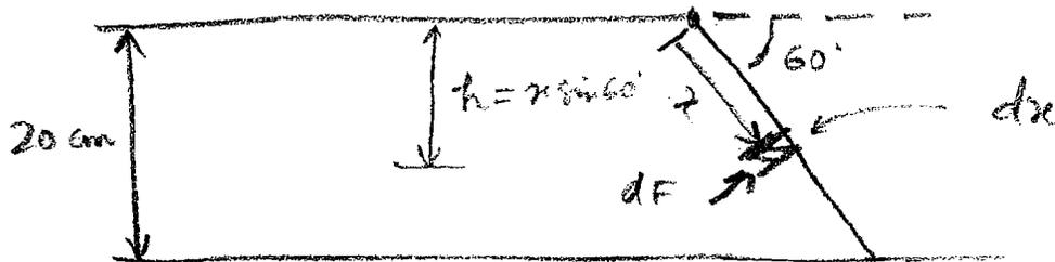
Consider a small element of thickness  $dx$  at distance  $x$  measured along the wall from free surface. The pressure at this element is
