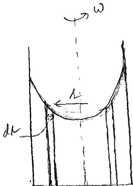
Consider a hollow cylindrical water surface of radius  $r$  thickness  $dr$  and height  $y$ .
