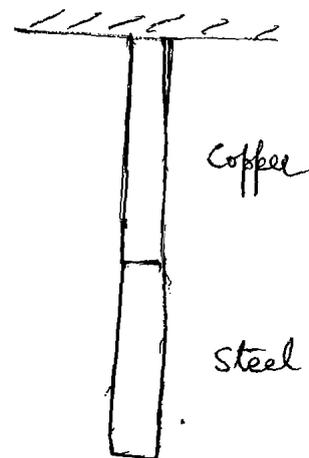
$$\Delta l_s + \Delta l_c = 0.7 \text{ mm} = 0.7 \times 10^{-3} \text{ m}$$
