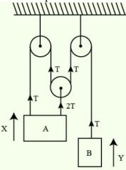
Using work done by tension method, (net work-done by tension is zero, since it is internal force)
